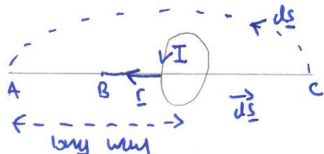
at A (large distance)  $R_A = 0 \rightarrow$  no change loop gain a  $\Omega$  of  $-2\pi$  ( $d\underline{s} \parallel -\underline{r}$ )  $\therefore$  at C net  $\Omega$  gain is  $-4\pi$ . Now along return path assume big  $\Omega$  so  $\Omega$  is not changed. Hence  $\int d\Omega = -4\pi \Rightarrow \int d\phi_m = \frac{I}{4\pi} \int d\Omega$
