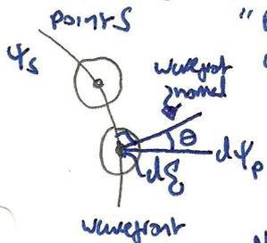
"Each unobstructed element  $dg$  on a wavefront at  $u$  gives instant acts as a source of secondary wavelets  $d\psi_p$  with the same temporal dependence as the primary wave  $\psi_s$ "
