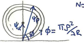
Note for unobstructed incident waves  $\psi_p = \psi_u$  corresponding to  $\rho = \infty$ . when  $\phi = n_{\text{odd}} \pi$   $\psi_p = 2\psi_u$ . (until  $k|\theta|$  becomes significant for high angles).  $< 1$ .
