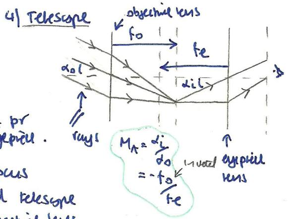
Note: If rays starting thin lens will meet at same place in the focal plane of the lens. For microscope and telescope treat focused image from objective lens as object for eyepiece lens.
