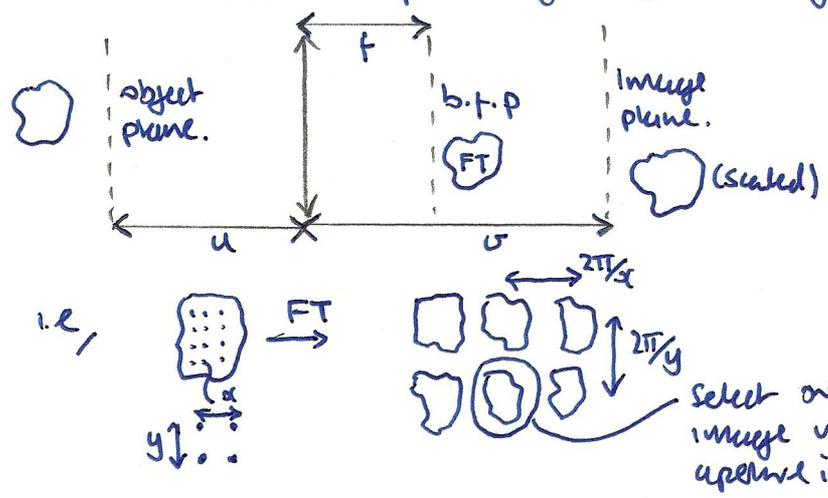
Note we can exploit this fact by filtering periodic functions in the object i.e. line lines in a TV picture via selecting proportions of construction images in the b.f.p.
