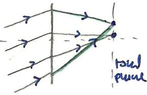
4) Astigmatism - cone of rays leaving a point on the object which is off axis will strike the lens asymmetrically - results in a focus in the vertical and horizontal directions lying in different focal planes.
