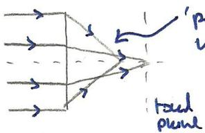
'peripheral' rays are focused before paraxial length - length appears to have higher power than it should. corrections: \* aspherical lens \* include a diverging lens into system \* reduce lens aperture size.
