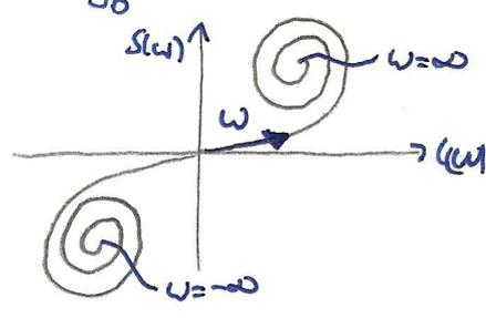
i.e.  $\psi_p$  is a spanning vector between  $\omega$  points on the spiral. i.e. Cornu spiral is an amplitude / phase diagram. i.e.  $\psi_p$  gives amplitude  $\psi_p$  phase  $\theta$ .
