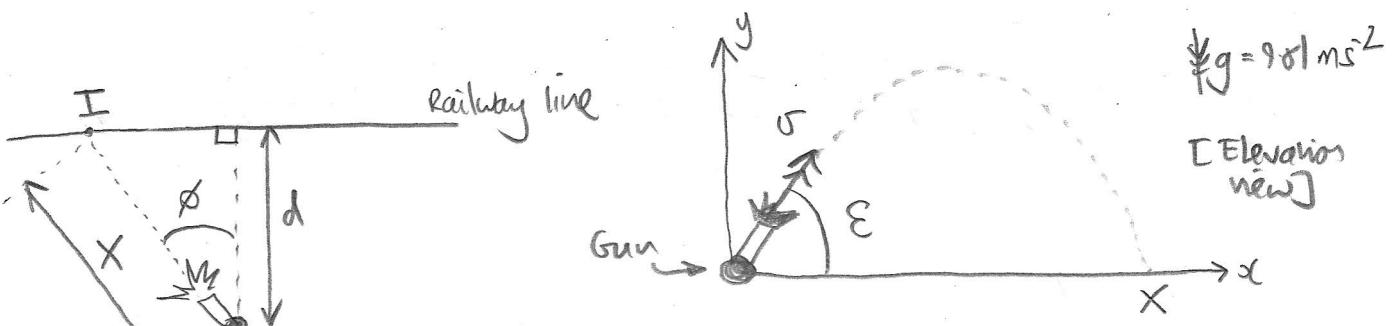
[Plan view] aim is to maximize time of flight such that the shell fired from the gun hits the railway line at I. Assume only gravity acts upon the shell (i.e. ignore air resistance) and the shell leaves the gun with speed  $v$ . Let time of flight be  $T$ .
