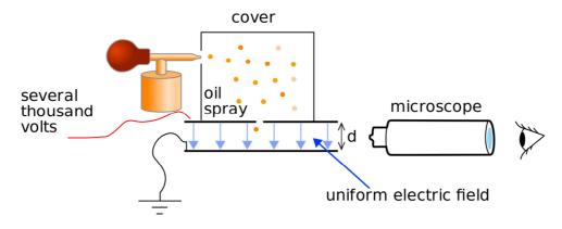
Figure 7. Millikan oil drop experiment apparatus (schematic). Source: <u>https://en.wikipedia.org/wiki/Oil\_drop\_experiment</u>
