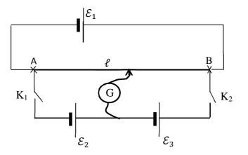
Figure 2(a). Cells connected to a resistance wire.
