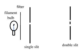
Figure 3(b). Filament bulb and single slit to illuminate the double slit.
