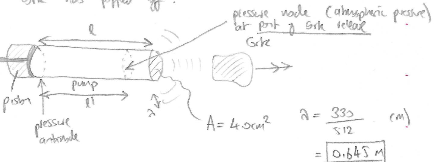
Pressure wave in tube at fundamental frequency has a pressure antinode at piston end and node (atmospheric pressure) at the open end  $\leftarrow$  when the cork is released! So  $l' \neq l$ .
