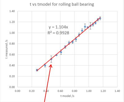
Error bars (in measured time) calculated from the standard deviation of the five timings.
