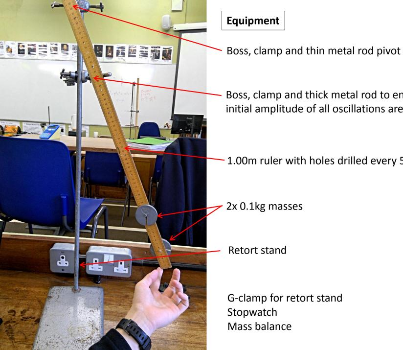
Boss, clamp and thick metal rod to ensure initial amplitude of all oscillations are the same
