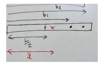
$$\overline{x} = \frac{M \times \frac{1}{2}L + mb_1 + mb_2}{M + 2m}$$
