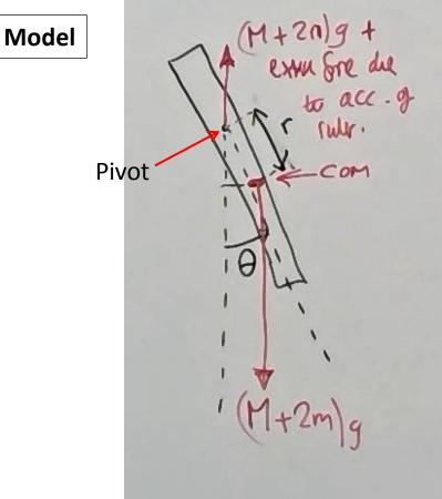
$$I\ddot{\theta} = -\underbrace{\left(M + 2m\right)g}_{\text{weight}} \times r\sin\theta_{\text{⊥distance}} \qquad \theta \ll 1 \text{ radian} \Rightarrow \sin\theta \approx \theta$$
