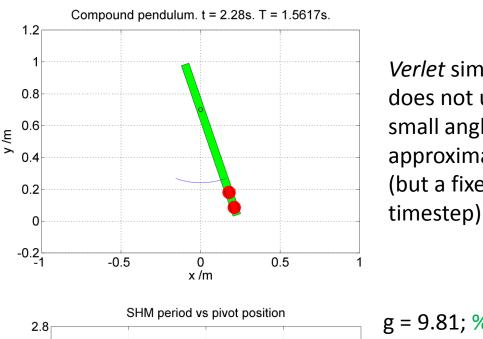
Ruler oscillation. T = 1.5617s. a = 0.3m. 0.4 SHM Verlet 0.3 Verlet simulation 0.2 Angle of rotation /rad does not use the small angle approximation (but a fixed -0.2 -0.3 -0.4<sup>L</sup> 5 15 10 time /s
