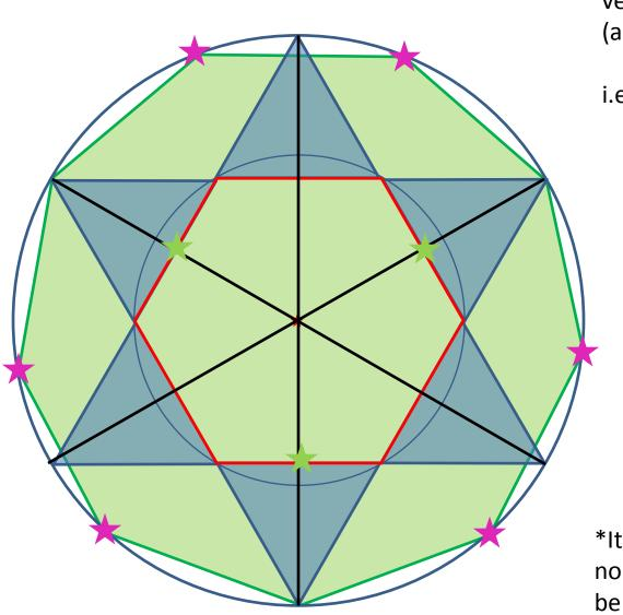
9. Connect up the arc intersections with three of the hexagram vertices to construct an (approximate) nonagon\*
