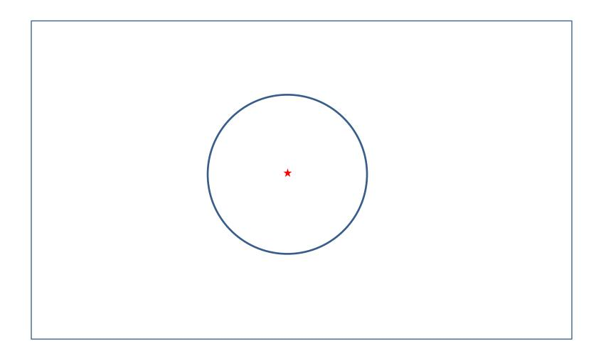
2. Without changing the opening angle of the compass, 'walk' it round the circle and hence construct a regular hexagon.
