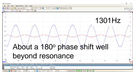
For **phase measurements**, drag a box in IrfanView between trough and peak of the  $V_0$  trace. Record number of pixels for 180° of phase (look in the title bar).
