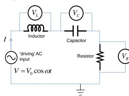
$$\frac{d^2 I}{dt^2} + \frac{R}{L} \frac{dI}{dt} + \frac{I}{LC} = \frac{-\omega V_0}{L} \sin \omega t$$
