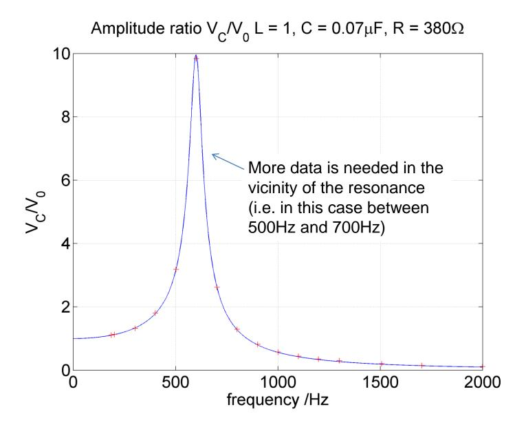
Data from Excel sheet overlaid upon a model curve. Computations and graphics production done via a MATLAB program lcr.m
