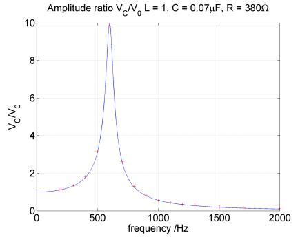
An LCR circuit is a single current loop which consists of an Inductor (essentially a coil of wire), a Capacitor (plates to store charge separated by an insulator) and a fixed resistor.
