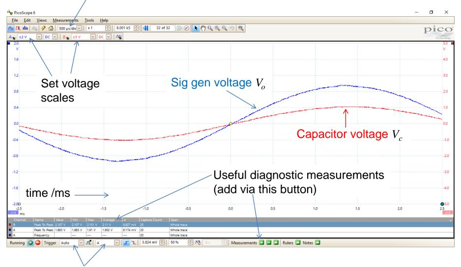
Set Trigger to be Auto, on source A (i.e. signal generator)
