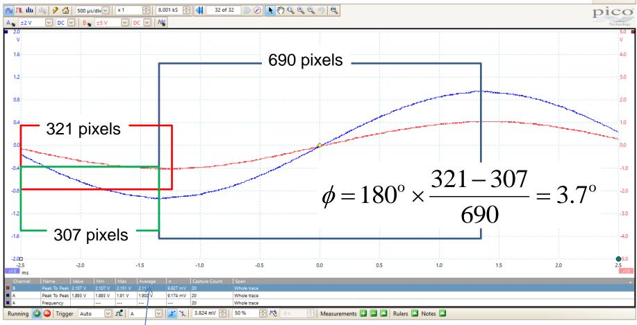
For amplitude measurements, simply halve the 'Peak-to Peak' values for each trace
