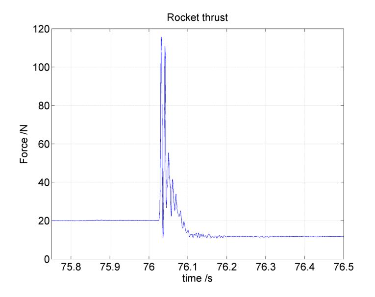
Force vs time during launch event (close up). Significant mechanical oscillations observed due to the 'impulse response' of the see-saw rig
