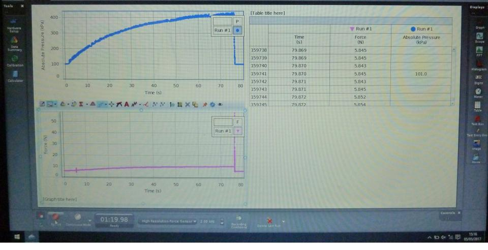
**Pressure vs time** and **Force vs time** traces in CAPSTONE software. To export data, select all data in the table, copy to the clipboard (ctrl+C) and paste into a text editor such as **Notepad**. This file can then be imported into **MATLAB**. Note there will likely be too many data points for Excel to handle! No. No. of Concession, Name
