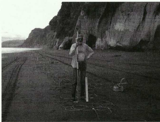
Figure 3.9: Staff mounted prism used to reflect the rangefinding laser.
