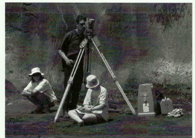
Figure 3.8: Tripod mounted theodolite and laser rangefinder are used to survey shot and geophone positions.
