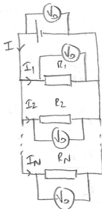
Each resistor is connected to the same cell, so "feels" the same electric field and  $\therefore$  PD across each bop is  $= V_i$ .
