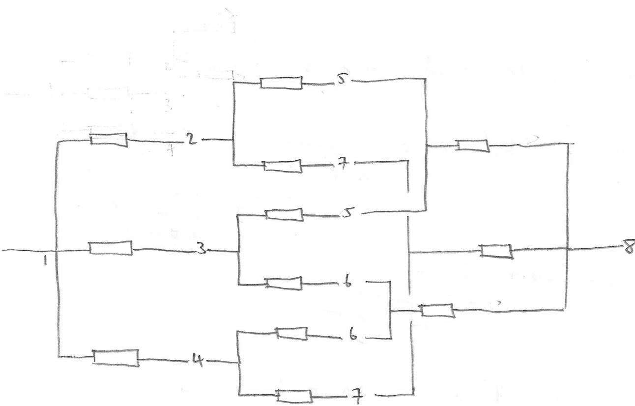
Now this is tricky to consider as a connection of parallel circuits because of the way the second set of vertices cross-link.
