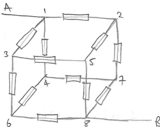
Consider a cube of identical resistors. Each has a resistance of  $1R$ .
