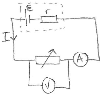
Power dissipated in variable resistor  $R$
