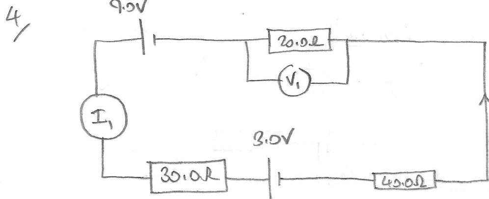
$$kI: \quad 9.0 - 3.0 = I_1 \times 30.0 + I_1 \times 40.0 + I_1 \times 20.0$$
