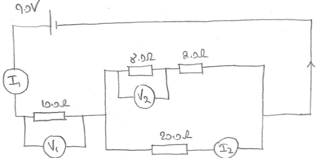
$$\begin{aligned} \text{Total resistance is: } R &= 10.0 + \frac{1}{\frac{1}{8+2} + \frac{1}{20}} \\ &= 16\frac{2}{3}\Omega \quad (16.7\Omega) \\ &\quad \uparrow \\ &\quad \text{keep exact for flow on calc} \end{aligned}$$
