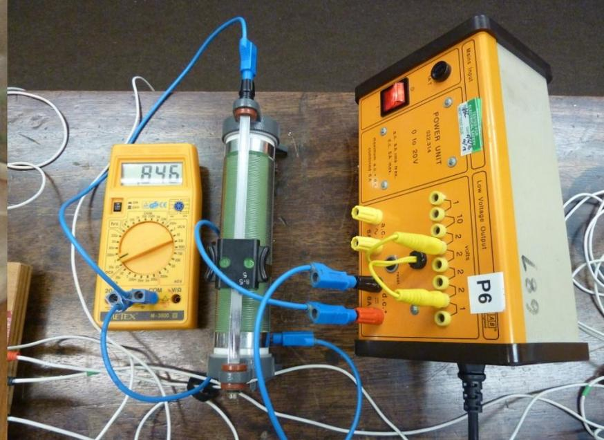
Helmholtz coil power supply & potentiometer. Current should be between 0.6 and 1.5 amps
