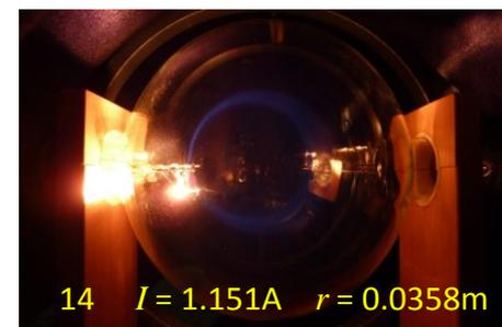
Using PowerPoint to measure beam radius  $r$
