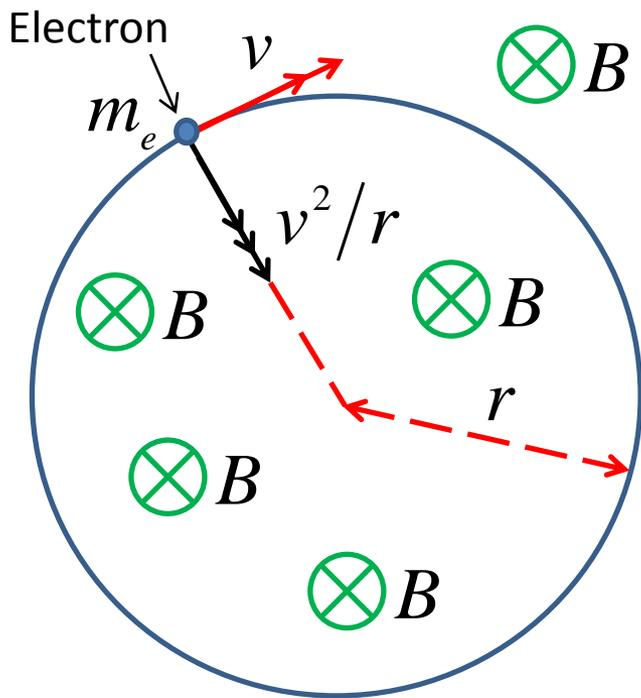
Assume *uniform* magnetic field of strength  $B$  between the Helmholtz coils.
