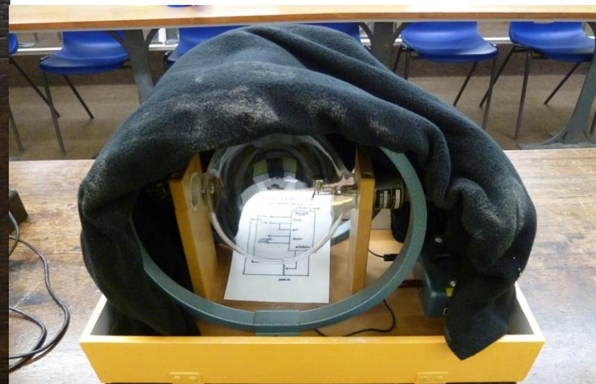
Fine beam tube + Helmholtz coils
