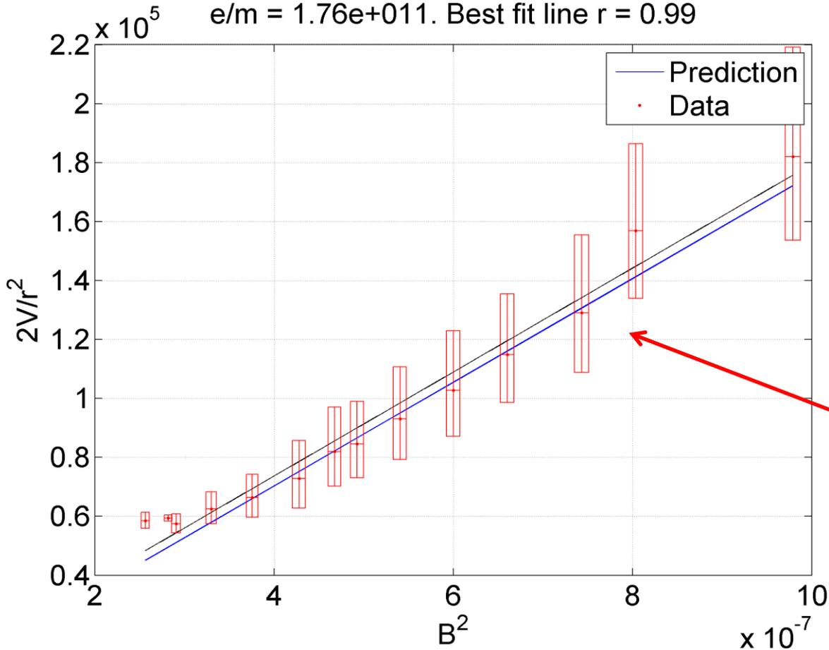
Fine beam tube experiment. Actual electron  $e/m = 1.76e+011$
