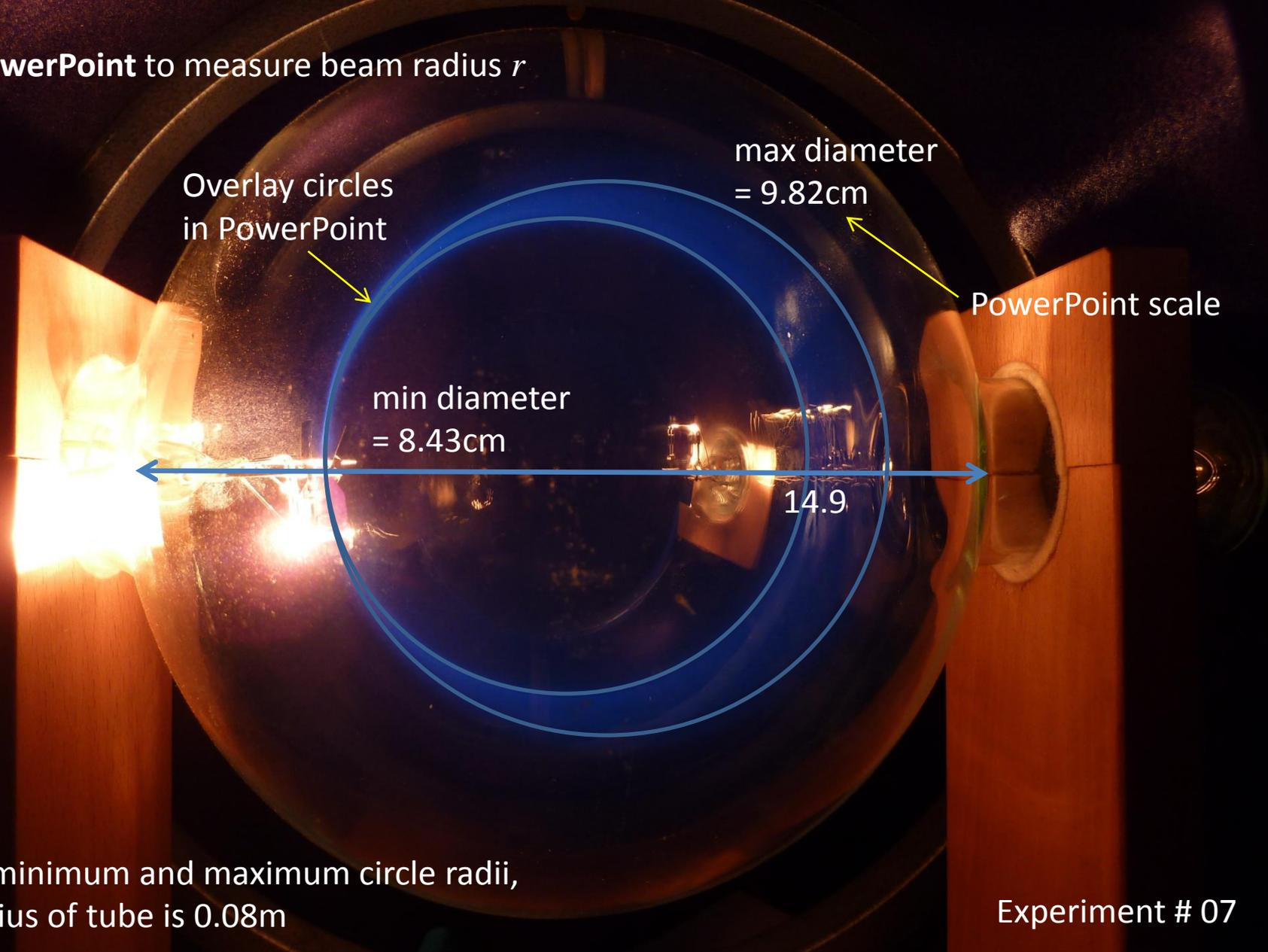
Calculate minimum and maximum circle radii, noting radius of tube is 0.08m
