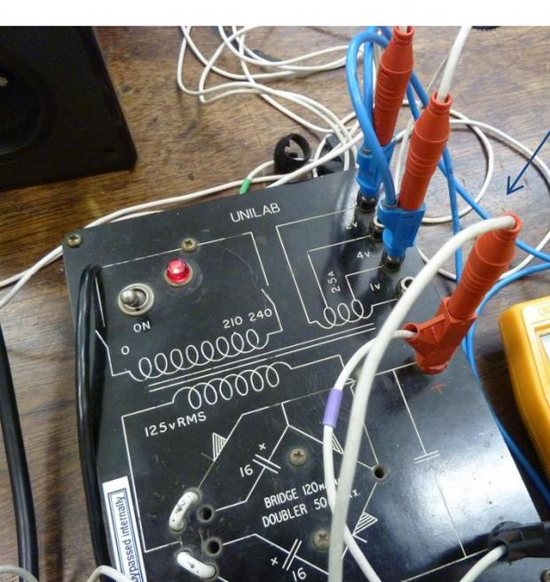
Checking the supply voltage before wiring up the Fine Beam Tube
