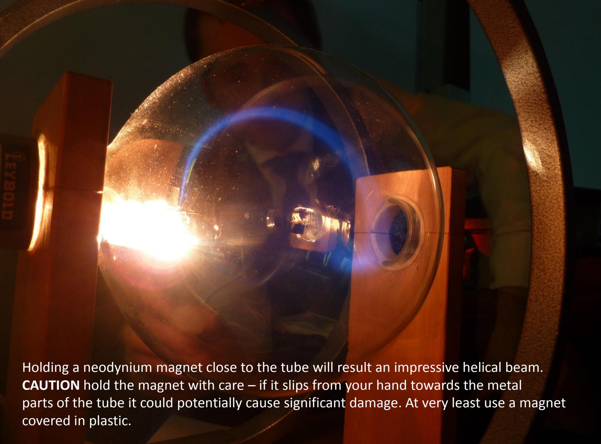
Holding a neodymium magnet close to the tube will result an impressive helical beam. **CAUTION** hold the magnet with care – if it slips from your hand towards the metal parts of the tube it could potentially cause significant damage. At very least use a magnet covered in plastic.
