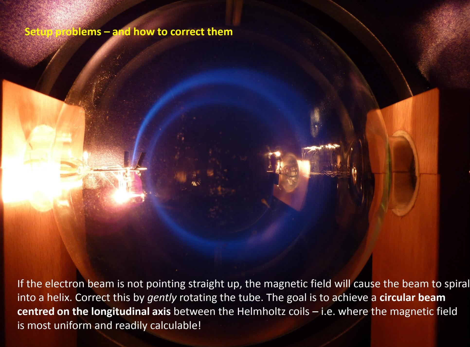
If the electron beam is not pointing straight up, the magnetic field will cause the beam to spiral into a helix. Correct this by *gently* rotating the tube. The goal is to achieve a **circular beam centred on the longitudinal axis** between the Helmholtz coils – i.e. where the magnetic field is most uniform and readily calculable!
