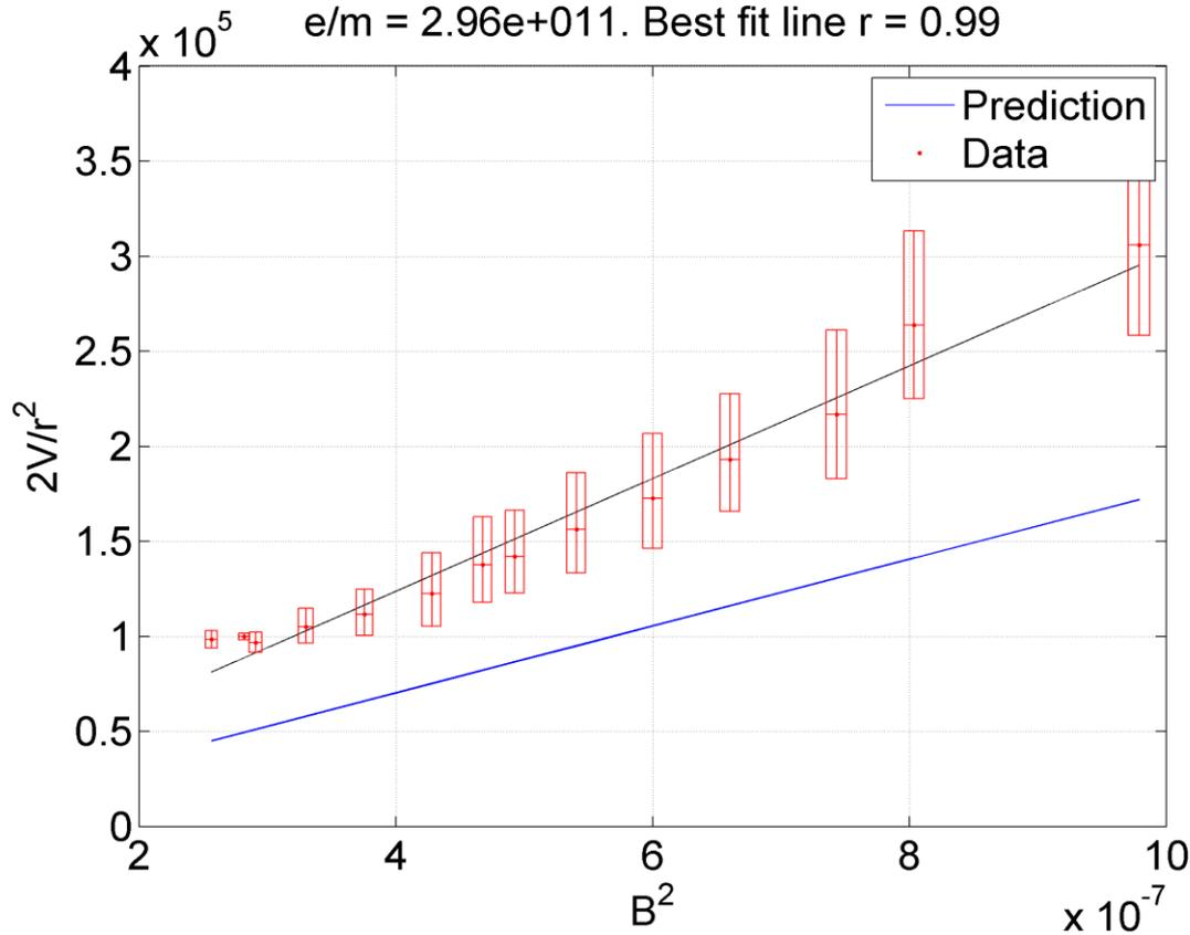
Beam radius is taken as the mean average of the max and min measured radii. The error is defined as half the difference between these radii.
