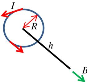
Magnetic field on axis from a current loop of  $N$  turns
