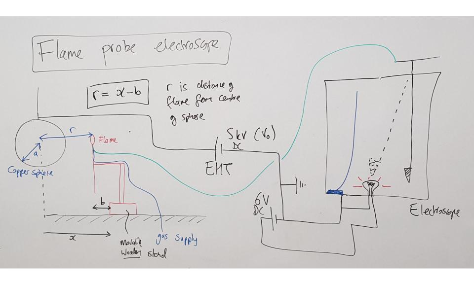
**Goal:** to show that the electric potential V varies *inversely* with distance r from the centre of an isolated charged sphere (when outside the sphere).
