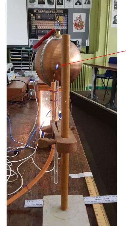
Align flame probe with centre of copper sphere.
