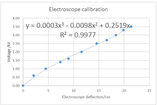
Photograph calibration and measurement electroscope deflection markings. Then measure off laptop screen and apply an empirical fit to determine the voltage.
