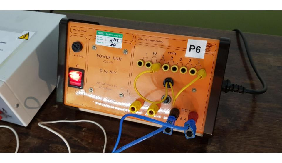
About 10V DC to light up the electroscope bulb
