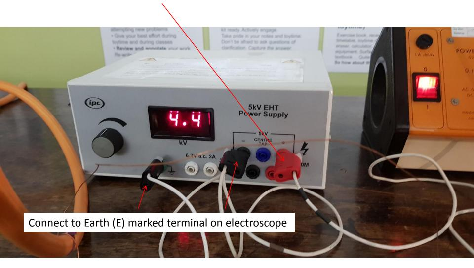
Don't connect across 10 mega-ohm resistors (i.e. the lower red and black terminals). The electroscope will leak charge a bit, and the charging time will be annoying long if you use the high resistances. You may find the electroscope needle can't maintain its position at a given flame probe position otherwise.
