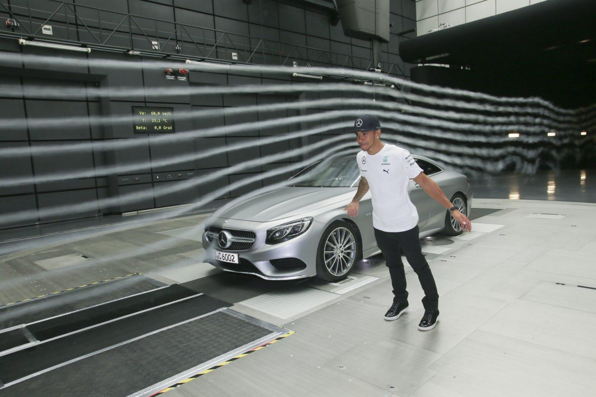
Aerodynamics of a sportscar (and driver!) being analysed using a wind tunnel
