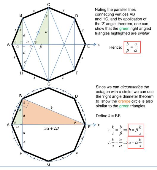
A volume of revolution of the octagon is the volume of **two cones** formed by the rotation of triangle ABH and **two frustums** formed by the rotation of trapezium BHGC
