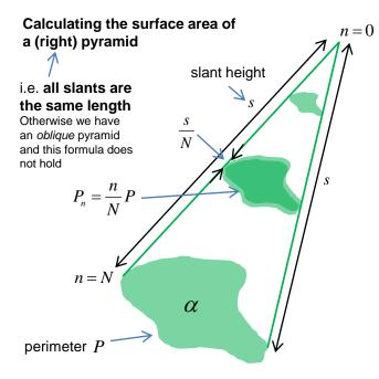
A pyramid of perpendicular slant height s and base perimeter P can be thought of being composed of an (infinitely) large number of **similar** *laminae*.
