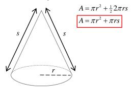
Note we can find the **curved area of a** *right* **cone** by noting how it can be constructed from a circle with a sector missing
