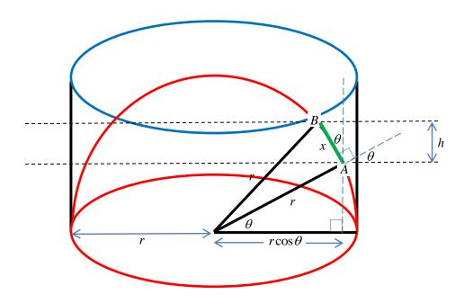
Consider the **tangent** to a circular cross section of a hemisphere at point *A*, which is at elevation angle  $\theta$  from the base of a hemisphere of radius *r*.
