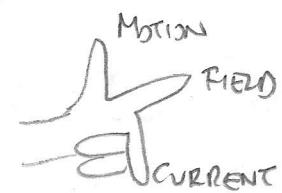
A time varying current through Al fil  $\Rightarrow$  an oscillation  $\perp$  to current and field, at same frequency as the AC (Alternating current).
