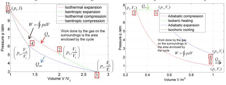
Example ideal heat cycles: A Carnot cycle (the most efficient, but difficult to achieve in reality), and a Diesel cycle.
