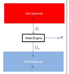
Work done compressing an ideal gas: dW = -pdV. Hence in differential form, the First Law is: dU = dQ - pdV. i.e. the change in internal energy equals the heat change of the gas + the work done on the gas. If the gas is compressed, dV < 0 which means the work done on the gas is positive. Note the work done by the gas (i.e. in a heat engine concept such as a petrol engine) is -dW = pdV.
