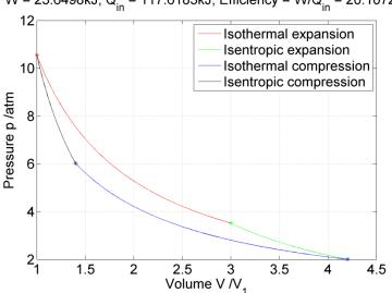
Carnot cycle:  $T_H = 100^{\circ}$ C,  $T_C = 25^{\circ}$ C,  $V_1 = 0.1m^3$ W = 23.6498kJ,  $Q_{in} = 117.6183$ kJ, Efficiency = W/ $Q_{in} = 20.1072\%$
