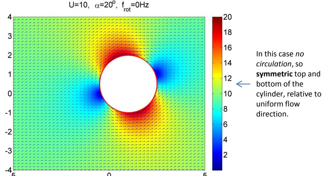
In this case no circulation, so symmetric top and bottom of the cylinder, relative to uniform flow direction.
