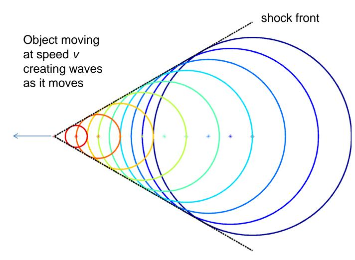
'Infinitesimally thin' spherical shells of disturbance are created continuously as the object moves. They radiate out at the wave speed *c*
