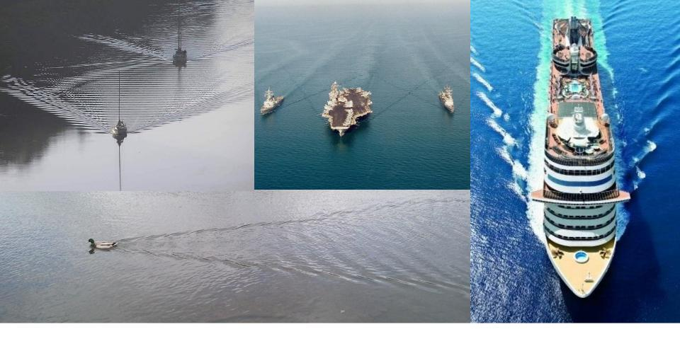
A wake is an *interference pattern* of waves formed by the motion of a body through a fluid. Intriguingly, the angular width of the wake produced by ships (and ducks!) in deep water is the same (about 38.9°). A mathematical explanation for this phenomenon was first proposed by Lord Kelvin (1824-1907). The triangular envelope of the wake pattern has since been known as the *Kelvin wedge*.
