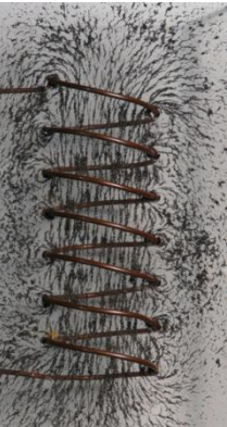
Magnetic field produced by a coil of current carrying wire. This is called a solenoid .
