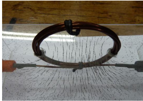
Iron filings aligning with a magnetic field generated by a few loops (a "ring") of current carrying wires
