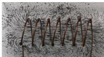
Solenoid magnetic fields are very similar to those of a permanent bar magnet
