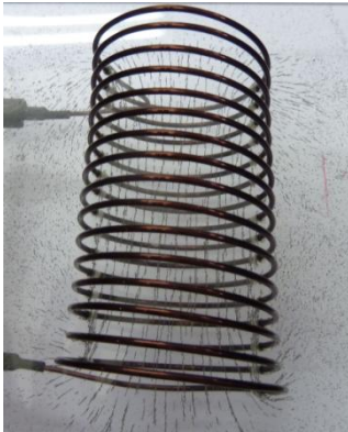
Magnetic field produced by a coil of current carrying wire. This is called a solenoid .
