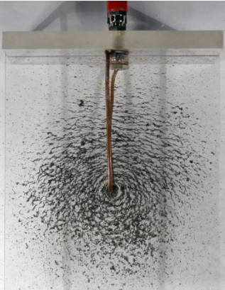
Iron filings aligning with a magnetic field generated by a current carrying wire
