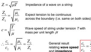
Wave speed of string under tension *T* with General result relating wave speed and impedance
