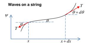
Consider an infinitesimally small section of a string of mass per unit length  $\mu$  under constant tension T
