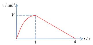
Between t=0 and t=1 seconds, acceleration a is  $a=a_0-At$  Cat is moving at constant speed at t=1  $0=a_0-A$   $\therefore a_0=A$
