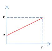
The acceleration is the gradient:  $a = \frac{v - u}{t}$   $\therefore$  v = u + at
