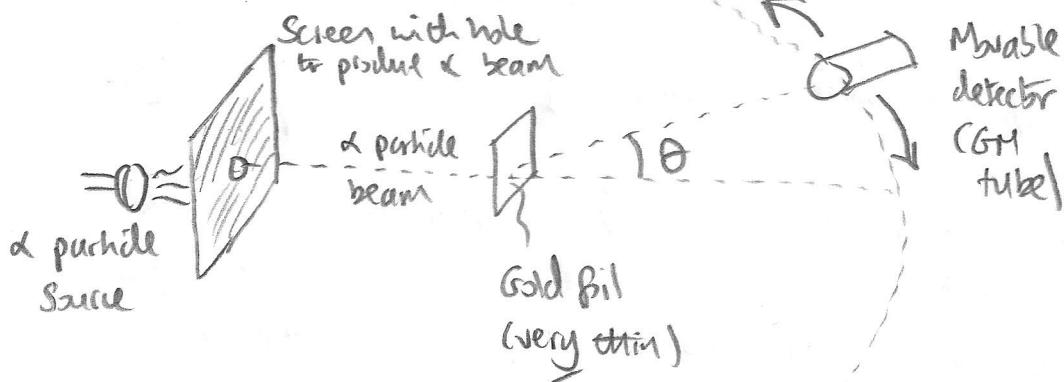
The experiment determined the statistics of scattered  $\alpha$  particles (He nuclei from radioactive decay) with angle  $\theta$ , by a very thin gold foil.
