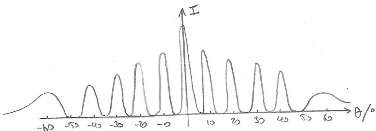
Note there will be some 'envelope' due to the finite widths of the 'slits' which produce the diffraction pattern.
