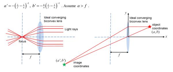
A projector has a focal length f of 20.0mm. An image of Christiaan Huygens of height 1.6m is projected on a screen 5.0m away from the lens. Determine the height of the (probably LED) light source corresponding to Mr Huygens, and also calculate how far away from the lens it is.
