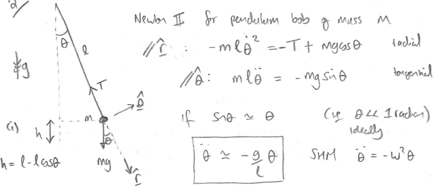
$$\text{so } \omega = \sqrt{\frac{g}{l}} \quad \therefore \frac{2\pi}{T} = \sqrt{\frac{g}{l}} \quad \therefore \boxed{T = 2\pi \sqrt{\frac{l}{g}}} \text{ period}$$
