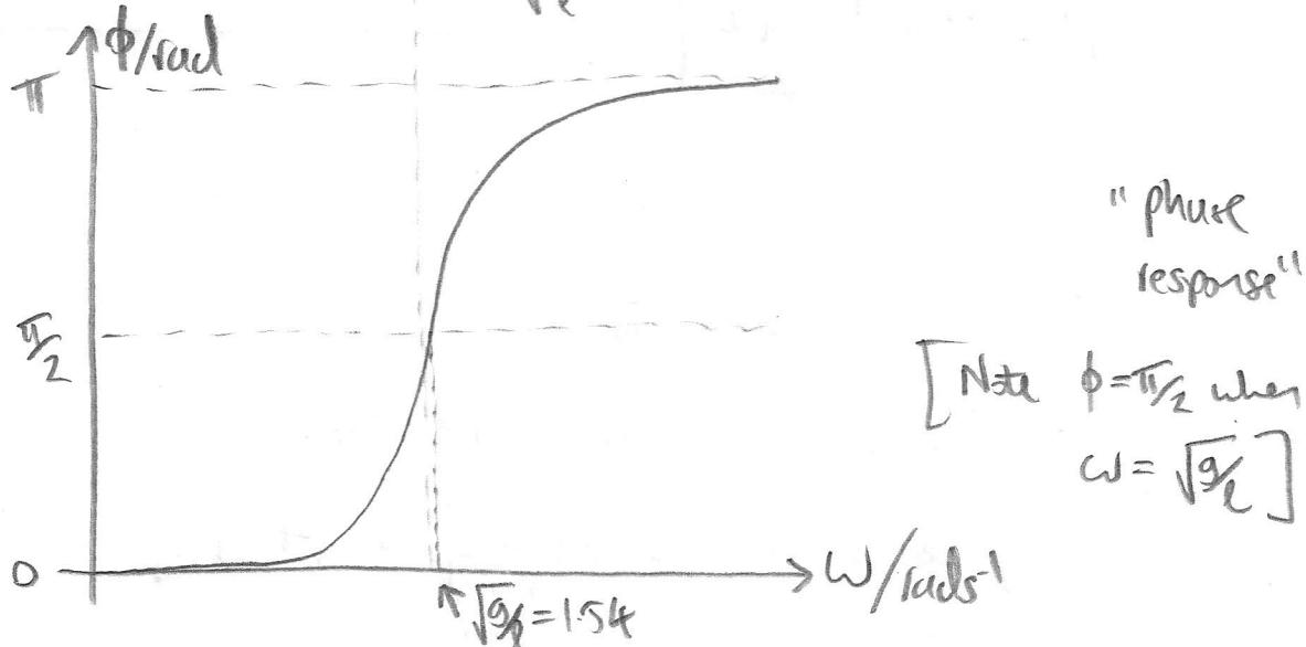
(ix) If the swing was critically damped  $\gamma = \omega_0$
