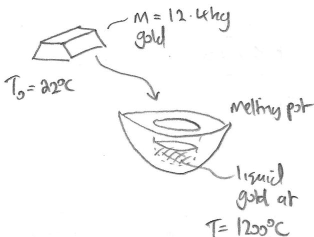
$$\Delta E = C_s M (T_{\text{melt}} - T_0)$$
