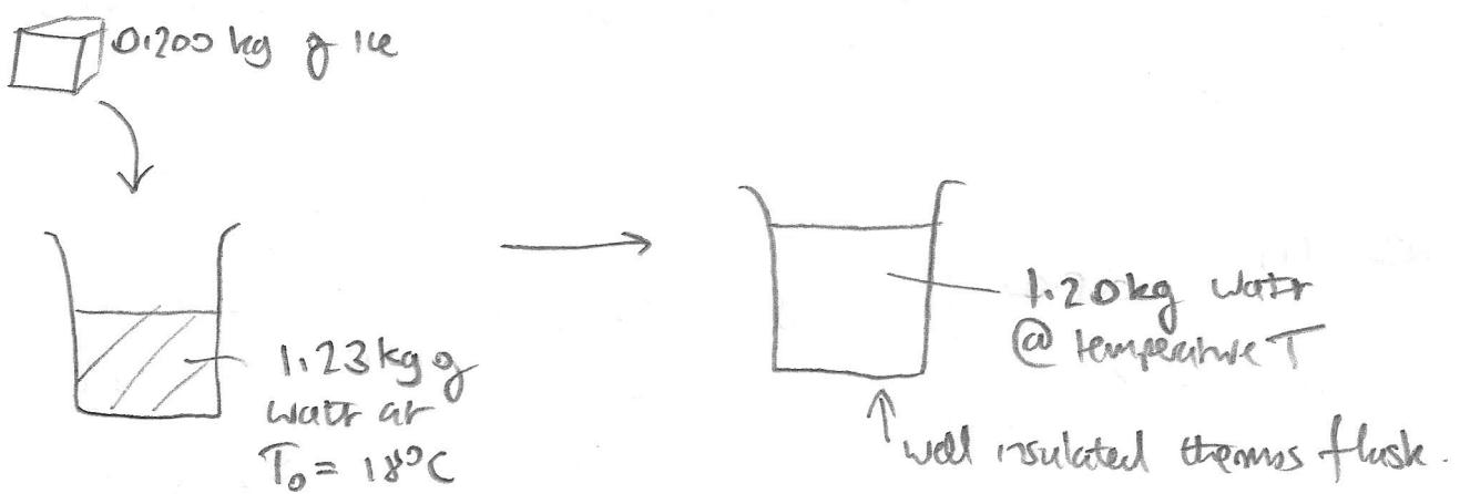
$$\text{Energy balance: } \underbrace{M_{ic} L_{fus}}_{\text{energy gain by ic}} + \underbrace{c_L M_{ic} T}_{\text{energy loss from water}} = c_L M_W (T_0 - T)$$
