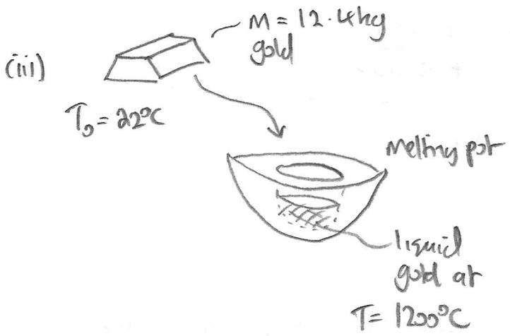
$$\Delta E = c_s m (T_{\text{melt}} - T_0) + mL_{\text{fus}} + c_L m (T - T_{\text{melt}})$$
