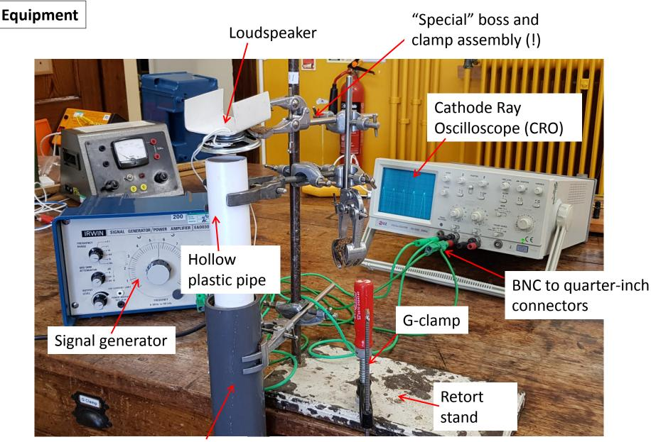
Plastic pipe filled with water (sealed lower end). Plus:
