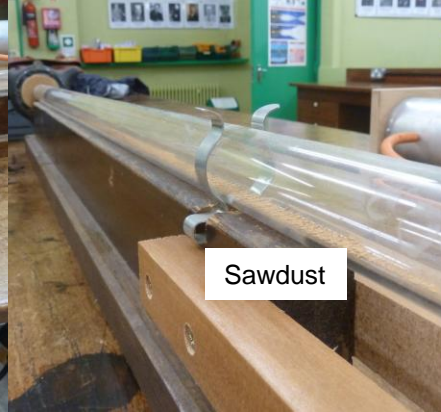
'Walls' of sawdust at displacement antinodes
