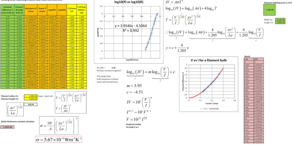
Interestingly, the  $\log_{10}(IV)$  vs  $\log_{10}(V/I)$  graph has a gradient much closer to 4 than 3.3. It appears that the resistance of the bulb is almost proportional to its temperature. Perhaps the assumption of all the electrical energy being radiated by the filament is flawed. There will inevitably some heat transfer into other parts of the bulb too, and indeed conduction into the low density gas within the glass bulb.
