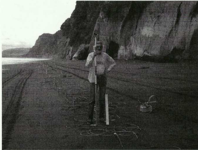
Figure 3.9: Staff mounted prism used to reflect the ranging laser.
