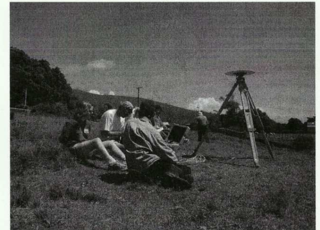
Figure 3.10: Global Positioning System (GPS) used to locate a fixed reference point from which all positions were calculated relative to.
