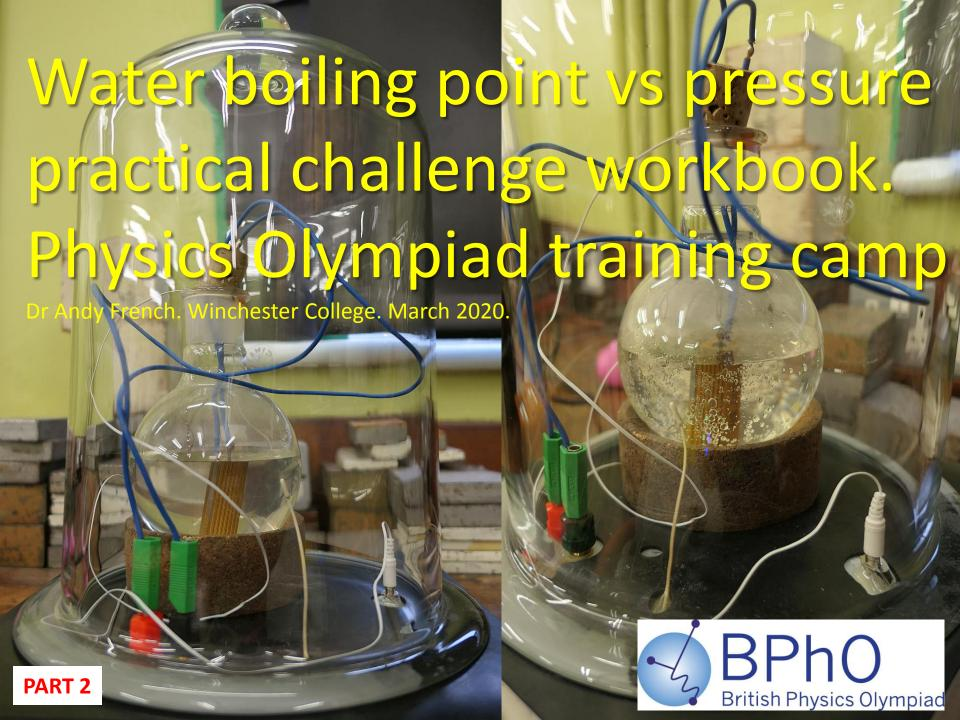
$$p(T_{boil}) = p_* e^{rac{L_{vap}}{RT_*}} e^{-rac{L_{vap}}{RT_{boil}}}$$
