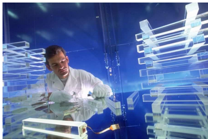
Scintillators made of \text{PbWO}_4 (transparent crystal) for the EM calorimeter of the CMS detector
